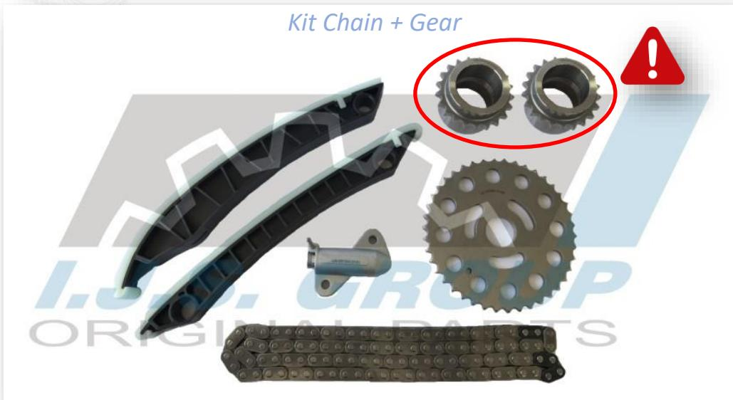
Check that the crankshaft gear you removed matches the equipment in this kit. If an incorrect crankshaft gear is installed, the crankshaft pulley will be misaligned preventing proper transmission of the auxiliary belts.
